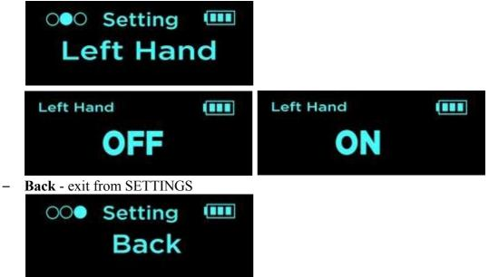
You use the MENU / PWR button to switch options. You enter an option by pressing the OK button. You dock changes in the option by pressing the + / 50 button or the - / 1k button. You save and exit the option by pressing the MENU / PWR button.
